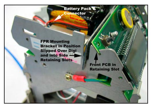
Figure 2-6. Front PCB & FPR Mounting Bracket in Position.
